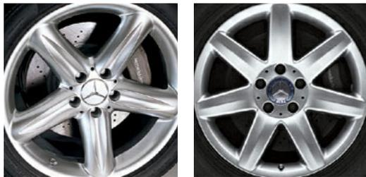
The SL 500 glides on striking new 18" 5-spoke aluminum alloy wheels with 255/40WR18 high-performance tires in front and 285/35WR18s in back. Or, if you prefer even smoother sailing, you can order your SL with the no-charge option of 17" 7-spoke wheels with 255/45WR17 high-performance tires.<sup>1</sup>
