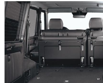
Here's one standard feature that actually gives you options. The second-row seats fold forward in a 60/40 split, so you can accommodate up to five passengers, or nearly 80 cu ft of cargo, or a variety of combinations in between.
