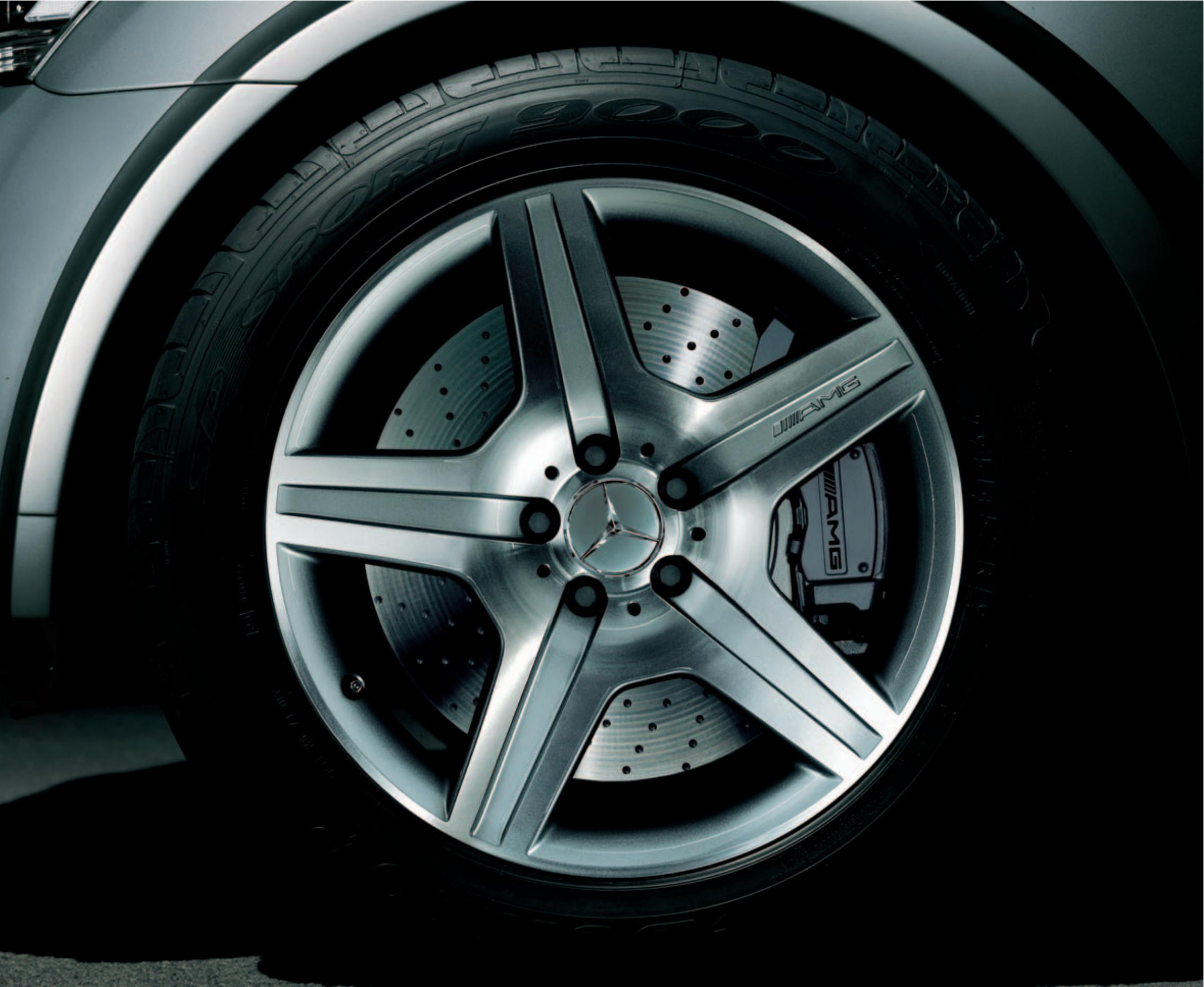
19-inch high-sheen AMG light-alloy wheels with 295/45 tyres, an AMG high-performance braking system with 2-piston sliding callipers and 390-mm internally ventilated and perforated front brake discs
