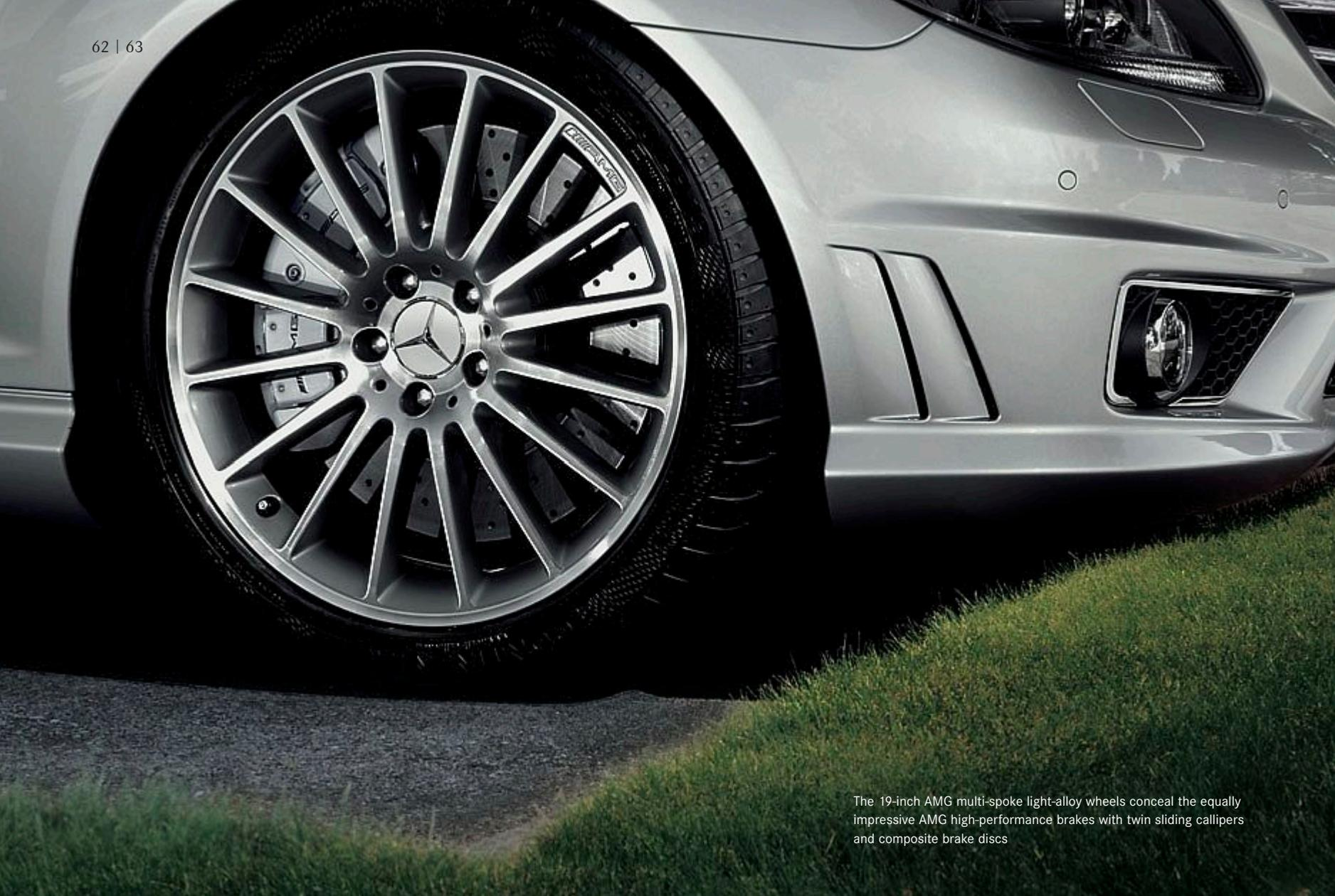
The 19-inch AMG multi-spoke light-alloy wheels conceal the equally impressive AMG high-performance brakes with twin sliding callipers and composite brake discs
