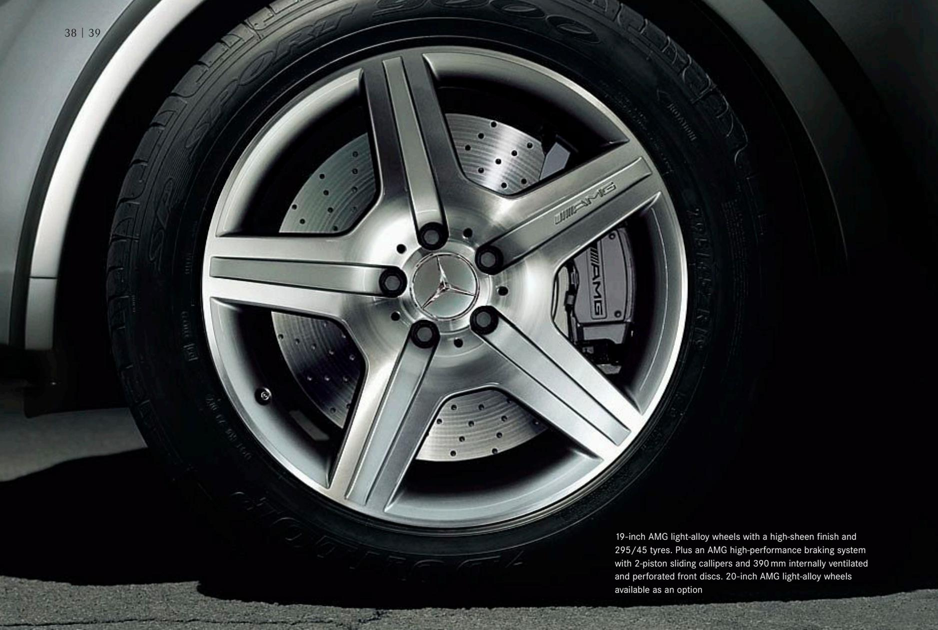
19-inch AMG light-alloy wheels with a high-shine finish and 295/45 tyres. Plus an AMG high-performance braking system with 2-piston sliding callipers and 390 mm internally ventilated and perforated front discs. 20-inch AMG light-alloy wheels available as an option
