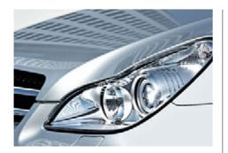
SHINING LIGHT THE INIMITABLY CURVED HEADLIGHTS LEAVE NOTHING TO BE DESIRED IN TERMS OF TECHNOLOGY – BI-XENON AND ACTIVE CORNERING LIGHTS GUARANTEE HIGHEST VISIBILITY IN ALL WEATHER
