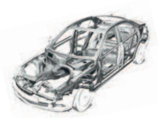
Before the new C-Class experienced an actual passive-safety crash test, it underwent some 5,500 digital tests on our supercomputers. For the sake of comparison, crash simulation models in 1989 were based on 26,000 elements. In sharp contrast, the new C-Class ensured far greater accuracy by incorporating 1.9 million.
