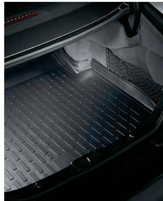
The non-slip flat boot tub is easy to clean and helps to protect the boot of your CLS
