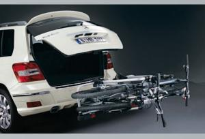
The laden bicycle rack can be pivoted downwards, allowing the load compartment to be opened
