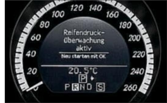
Tyre pressure loss warning system
