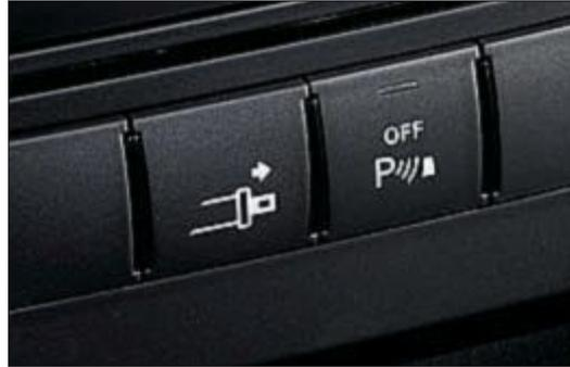
Button on centre console for belt feeder
