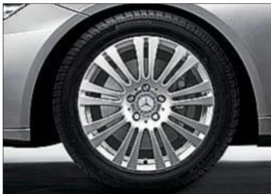
17-inch multi-spoke light-alloy wheel (standard for 4 and 6-cylinder)
