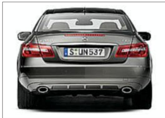
The 6-cylinder models are fitted with two oval tailpipes
