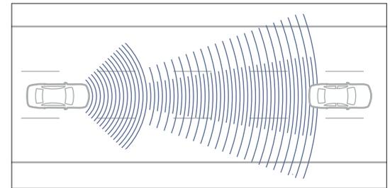
The DISTRONIC PLUS proximity control automatically keeps the coupé at a safe distance from the vehicle in front
