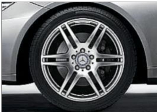
18-inch 6-twin-spoke AMG light-alloy wheel with mixed-size tyres (optional, Code 786, standard with the AMG Sports package)
