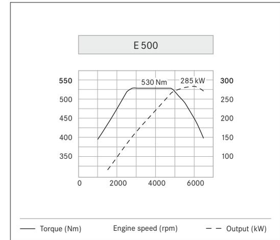
The E 500 places its impressive torque of 530 Nm at your disposal from 2800 rpm
