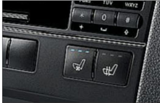
Climatised seats with button for seat ventilation/seat heating
