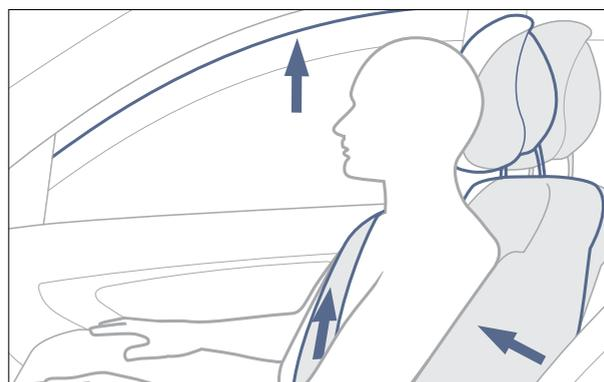
Should an accident be unavoidable; the GL-Class will automatically shut the windows, pull seatbelts tight and position the front seats for maximum safety.
