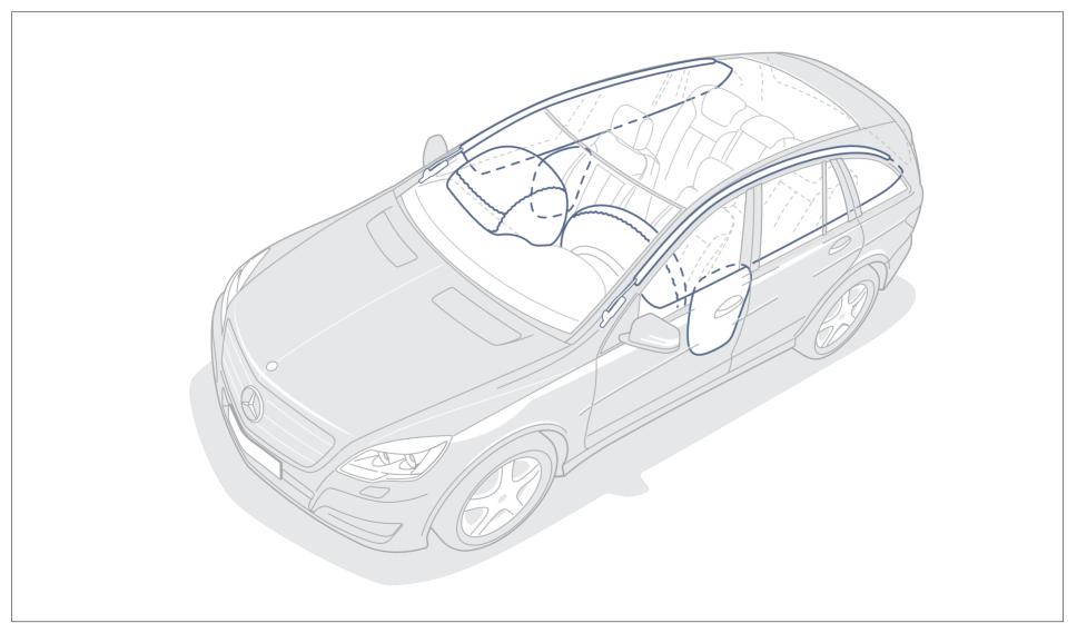
Eight-standard airbags including side curtain airbags in all three rows will support all occupants in the event of a vehicle impact.
