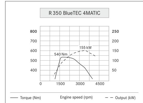
The R 350 BlueTEC 4MATIC achieves its maximum torque of 540 Nm as early as between 1600 and 2400 rpm
