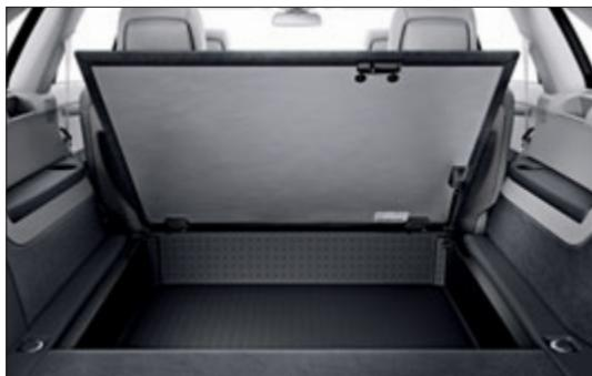
Stowage space beneath load compartment floor (for 5-seater)
