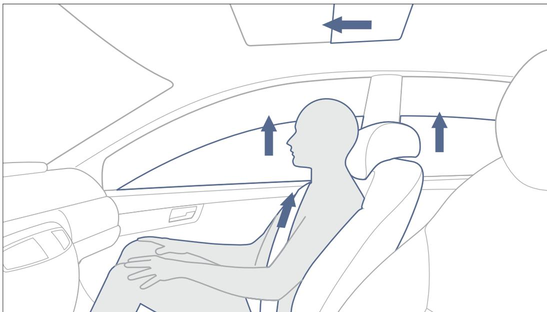
**PRE-SAFE® system** (standard). The anticipatory occupant protection system is able to detect certain critical driving situations in advance and activate preventive measures. If an imminent accident is detected, the system can close the side windows, move the front passenger seat to a more favourable position and tension the front seat belts automatically. It can also close the sliding sunroof, if fitted, and provide lateral support for the occupants if the multicontour seats are specified.
