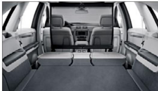
Safety and comfort rolled into one: optional partition net for occupant protection and load retaining
