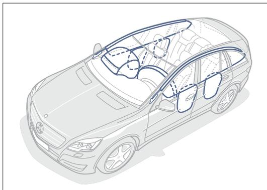
Standard equipment includes windowbags for all three possible seat rows plus airbags & sidebags for the driver & front passenger
